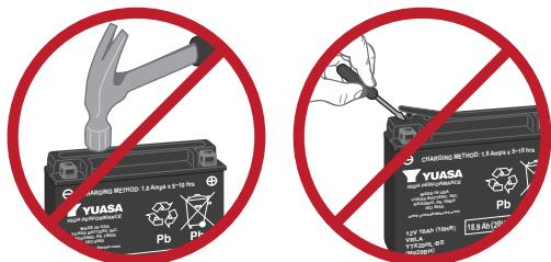
After filling, the sealing caps should be installed using hand pressure only. The sealing cap should never be removed once the battery is activated.
